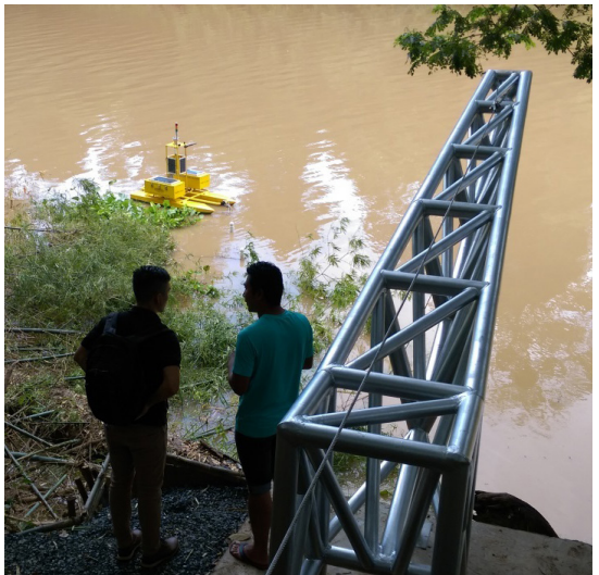
Figure 7: Custom support frame for high flow events
