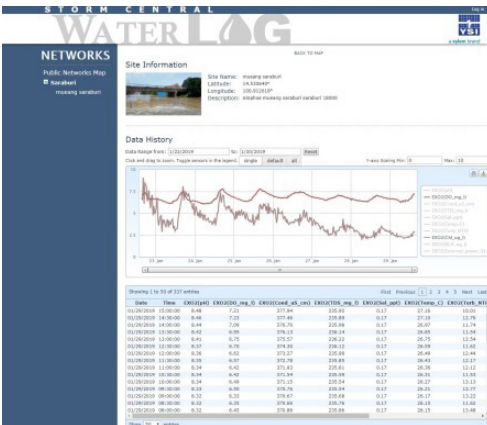
Figure 6: Storm Central real-time data display from the Station 5 Pisces buoy. Each site has a sign posted with project information and URL for public data access.
